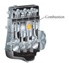
▲ The combustion of gasoline within an engine's cylinders does pressure volume work that ultimately results in the motion of the car.
