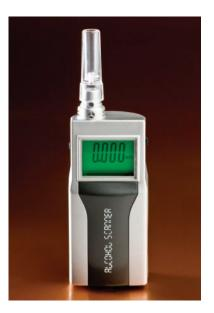
▲ FIGURE 20.19 Fuel-Cell Breathalyzer The fuel-cell breathalyzer works by oxidizing ethyl alcohol in the breath to acetic acid. The electrical current that is produced is proportional to the concentration of ethyl alcohol in the breath.
