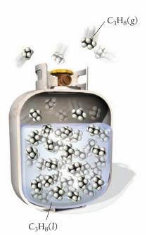
▲ The propane in an LP gas tank is in the liquid state. When you open the tank, some propane vaporizes and escapes as a gas.
