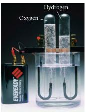
▲ Pure water is a poor conductor of electrical current, but the addition of an electrolyte allows electrolysis to take place, producing hydrogen and oxygen gas in a stoichiometric ratio.
