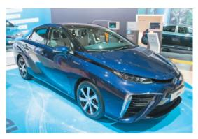
▲ The Toyota Mirai, a fuel cell vehicle that runs on hydrogen gas and produces only water as exhaust.
