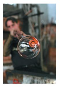
▲ Glassblowing involves blowing air into a hot piece of glass to form spherical shapes.
