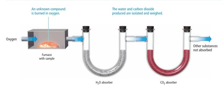
▲ FIGURE 3.13 Combustion Analysis Apparatus
